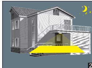
Lamp switches on 30% when natural light < 50Lux
